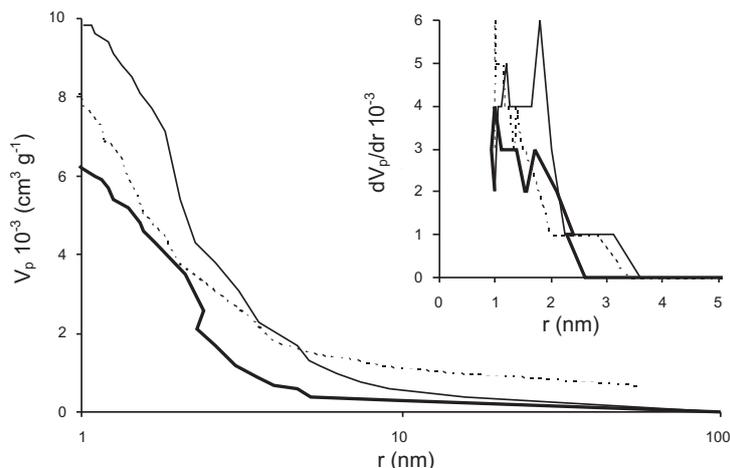
**Fig. 3.** Cumulative pore volume ( $V_p$ ) and differential pore size distribution (PSD) functions versus pore radius for rapeseed oil cake materials.
