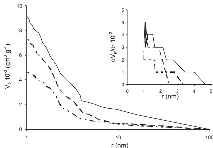
**Fig. 4.** Cumulative pore volume ( $V_p$ ) and differential pore size distribution (PSD) functions versus pore radius for rapeseed oil cake +wheat meal extrudate.
