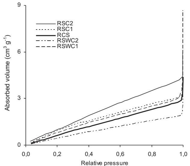
Fig. 1. Adsorption isotherms of nitrogen on the rapeseed oil cake and its mixtures with the wheat meal. Abbreviations: see in the text.
